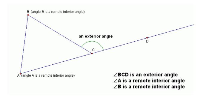
**Exterior Angle Theorem:** The measure of an exterior angle of a triangle is equal to the sum of the measures of the two remote interior angles.
